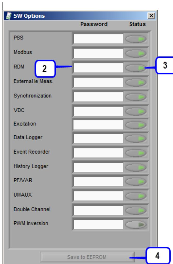
Figure 6-16. The SW Options window allows the user to enable optional software in the AVR.
