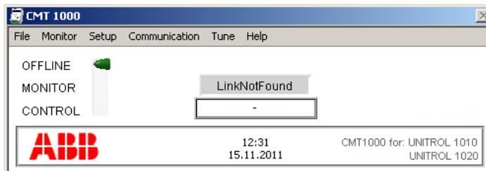
*Figure 6-11 LinkNotFound message when the AVR cannot be found or the communication port cannot be accessed by the CMT1000*
