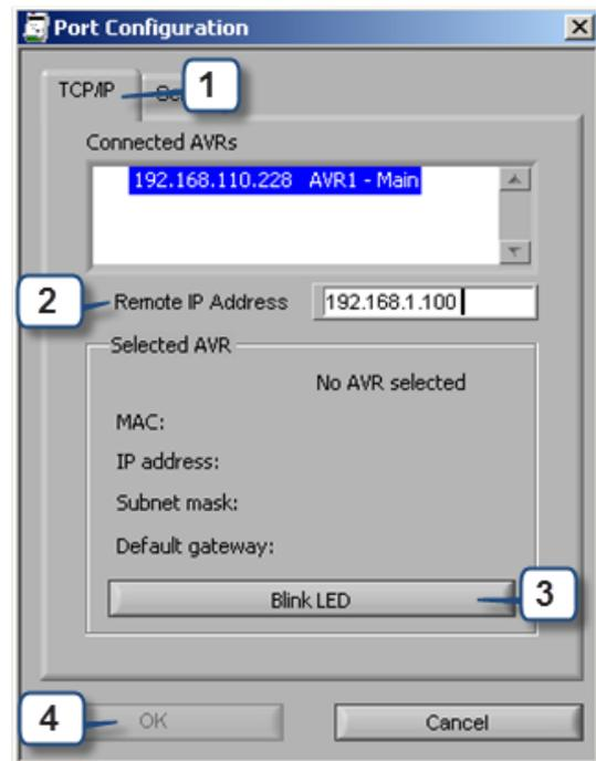
Figure 6-6 Remote IP Address Configuration.
