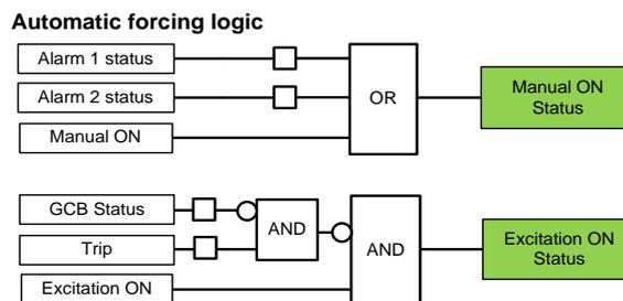
Figure 3-15 Automatic forcing logic
