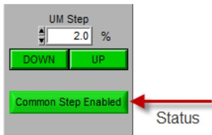
The common step function is disabled as soon as the mode is changed or the excitation is switched off.
