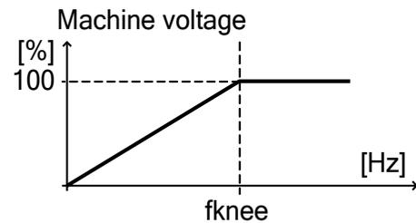
In case of a short circuit at the machine terminals, the frequency is calculated out of the machine current. This guarantees a correct functioning of the V/Hz limiter in any condition.
