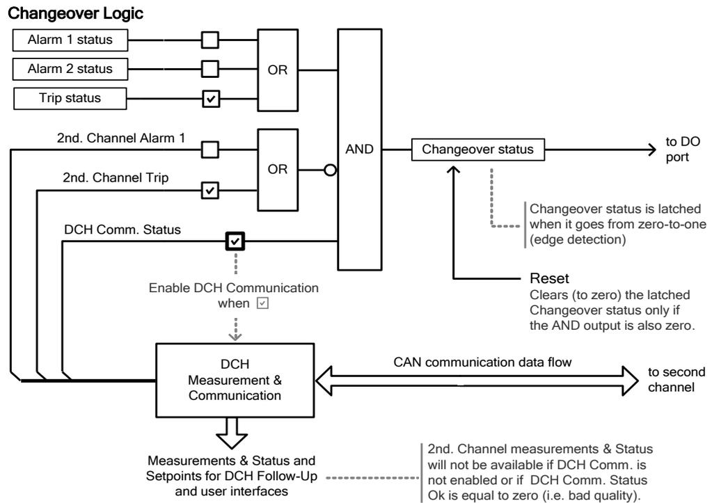
Figure 3-12 Channel Changeover logic and configuration.
