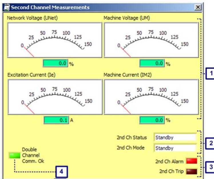
Figure 6-24 Second Channel Measurements window, when Double Channel communication over CAN is OK (data is being received correctly)
