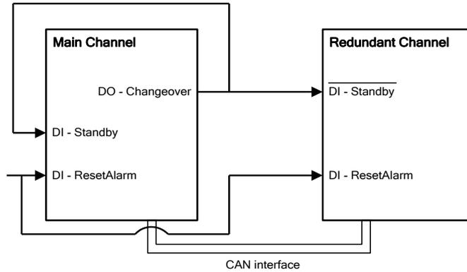
Figure 3-14 Typical configuration of Changeover output
