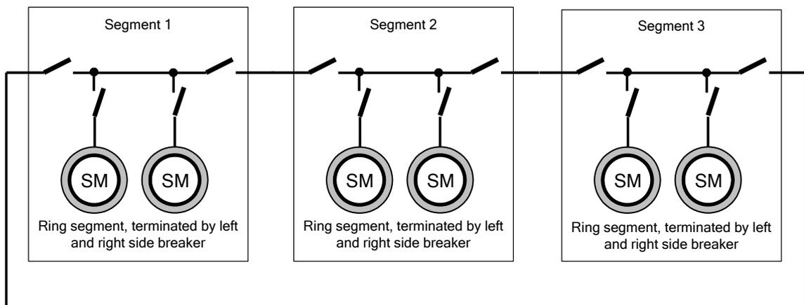
The auxiliary contact of the breaker must be wired only inside the segment. In order to select the correct machines regarding the load sharing, all AVRs give the information of the segment breaker and their own position (segment number) over the RS485 bus to all other AVRs. This enables the system to detect wrong configuration which is indicated as "VDC Ring Error".
