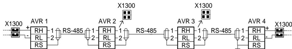
Figure 3-6 RS-485 wiring and jumper settings to use VDC on a set of four AVRs.
