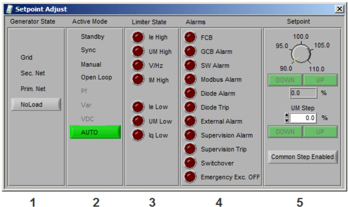
1. Displays the generator state condition, according to the Gen CB Closed and Parallel with the Grid status signals. Prim. Net and Sec. Net are used during VDC operation mode.
