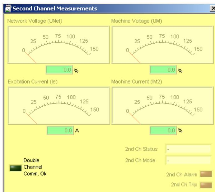
Figure 6-25 Second Channel Measurements, when Double Channel communication failed or is disabled.
