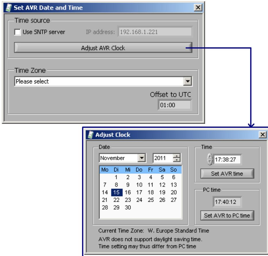
Adjust the time by means of the lower and raise buttons, then click Set AVR time
