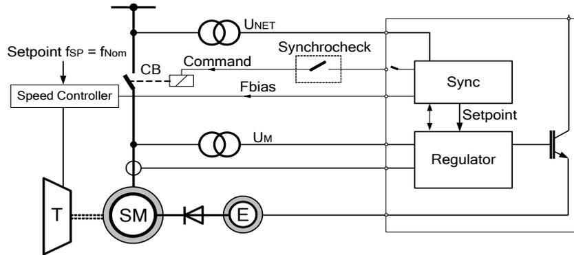
Figure 3-8 Typical application for Synchronization.
