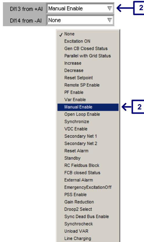
When using AI pins for DI signals, both inputs should not simultaneously be active.
