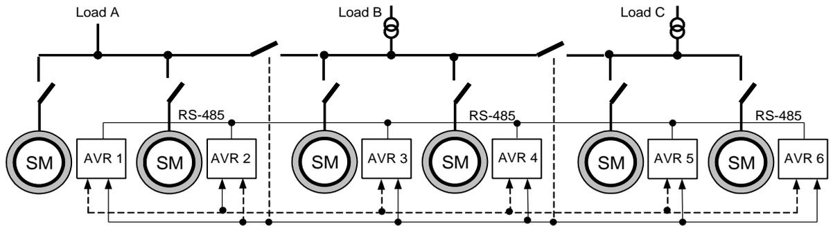
Figure 3-9 VDC application example of six machines and two nets.
