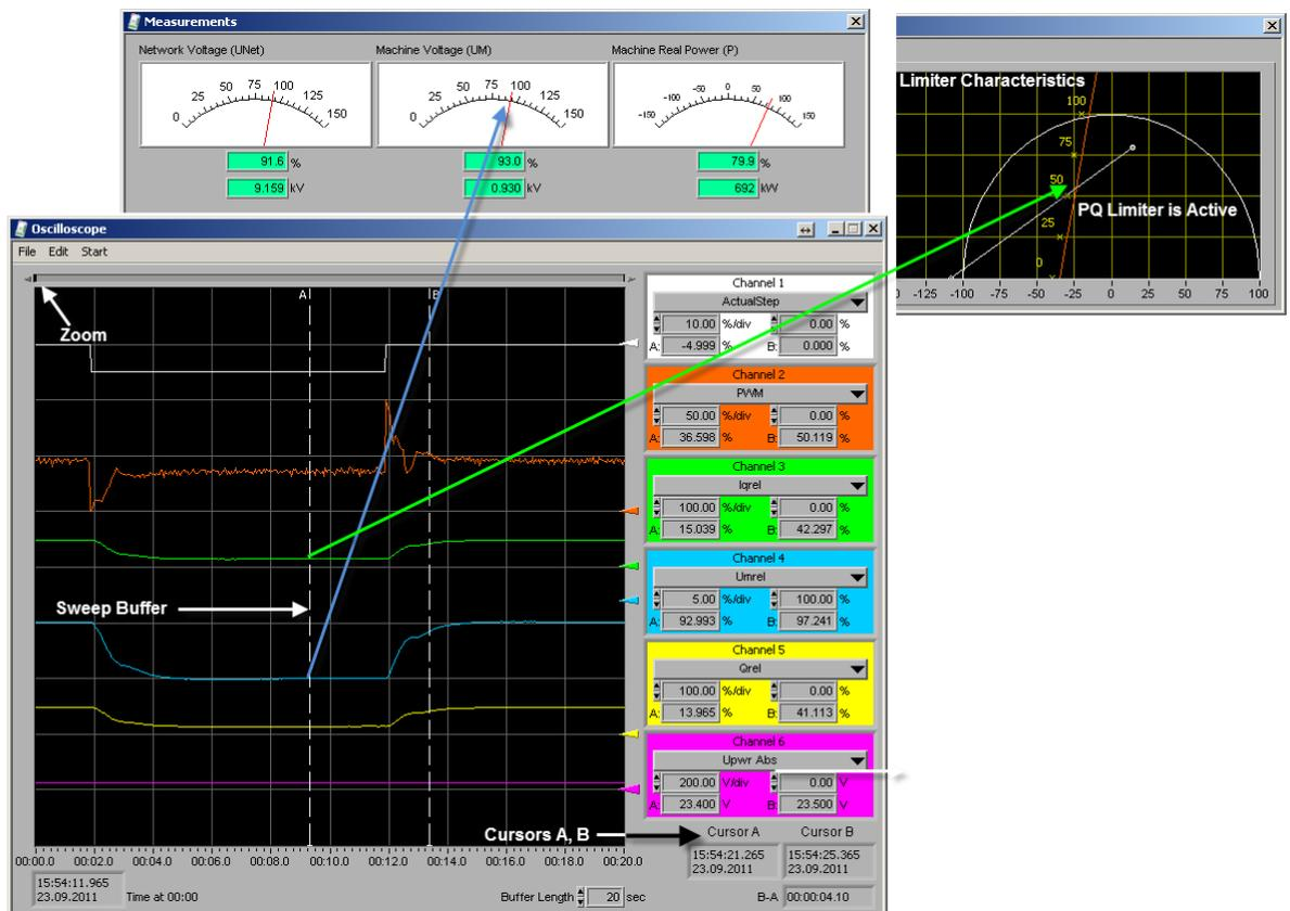
Figure 6-22 Evaluation of a waveform
