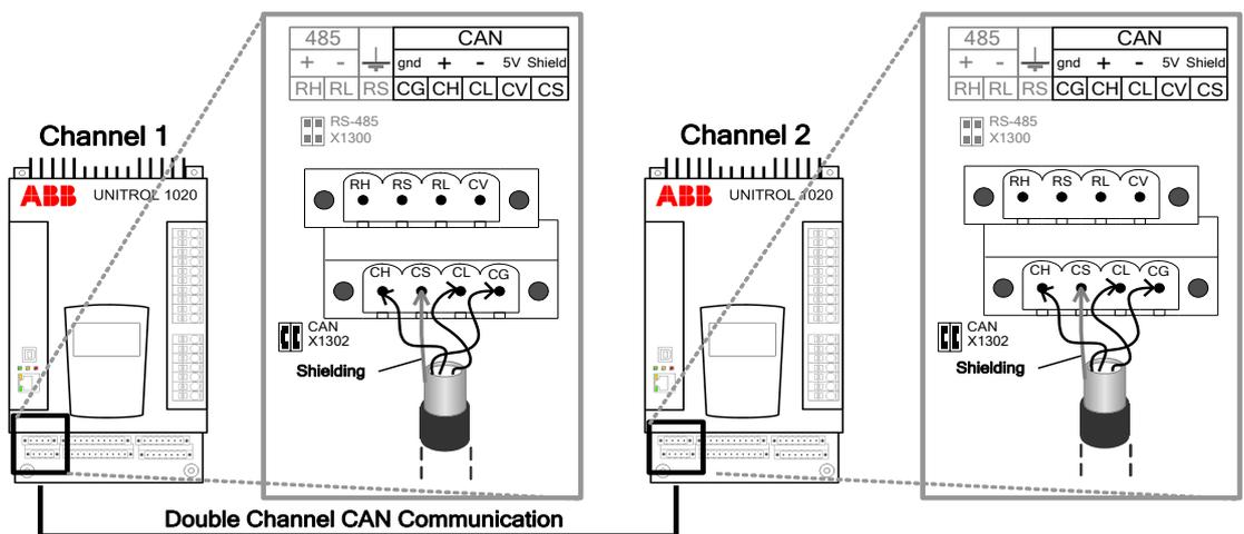
Figure 3-7 CAN connection for Double Channel SW
