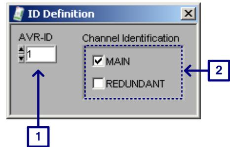
If the Double Channel feature is not used, the channel identification can be changed without affecting other UN1020 functions with the exception of the Modbus ID, which is used for CMT1000 access. That allows changing the name displayed in the CMT1000 and panel. For more information refer to Chapter 3.4.6 Modbus for Remote Access
