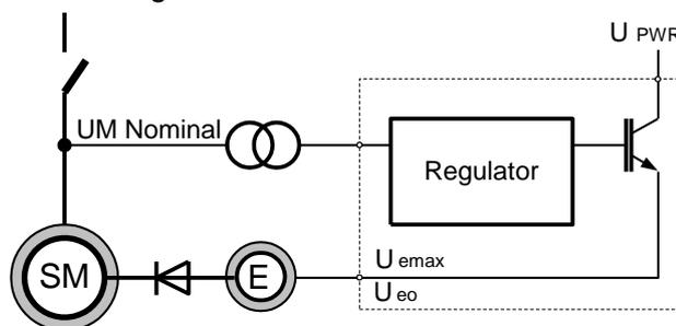
PWM no load: Regulator output at no load (PWM)
