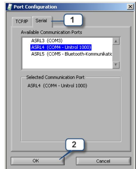
Figure 6-5 USB COM Port Configuration.
