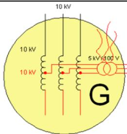
When the neutral point is opened, the transformer receives the full primary voltage and burns
