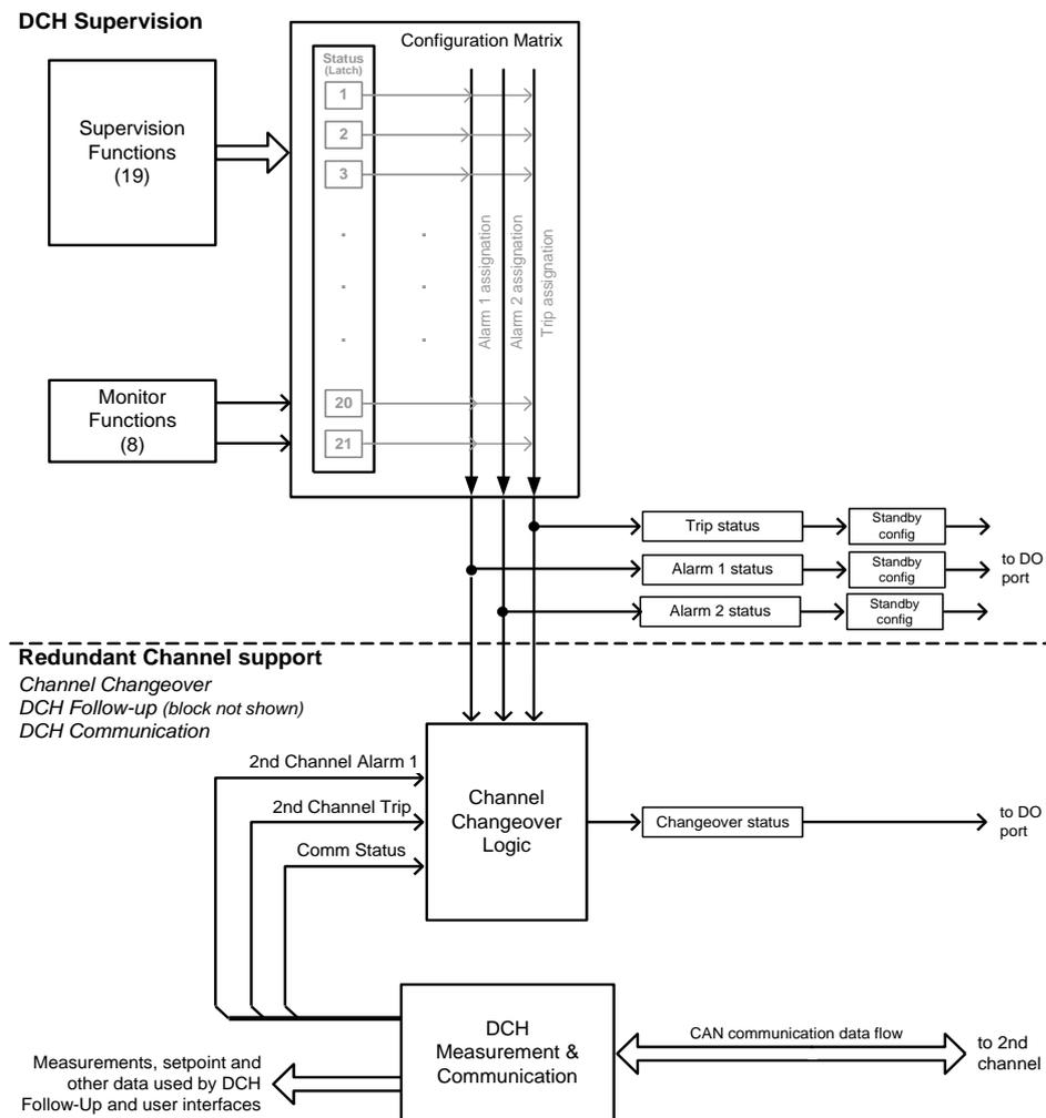
Figure 3-10 Schema of main Double Channel functions.
