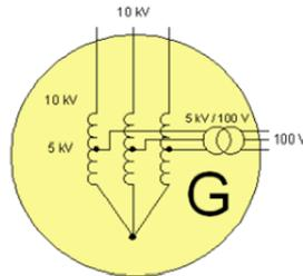
Generator transformers do not always measure the full primary voltage
