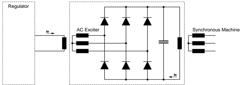
Figure 3-16 Rotating Diode Monitoring application
