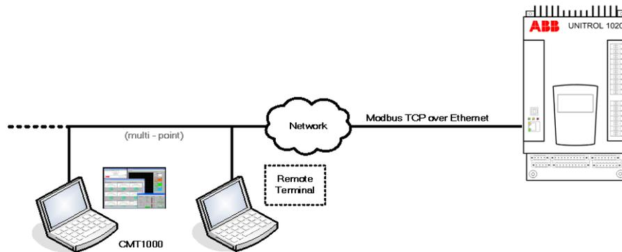
Figure 3-3 Ethernet TCP/IP connection
