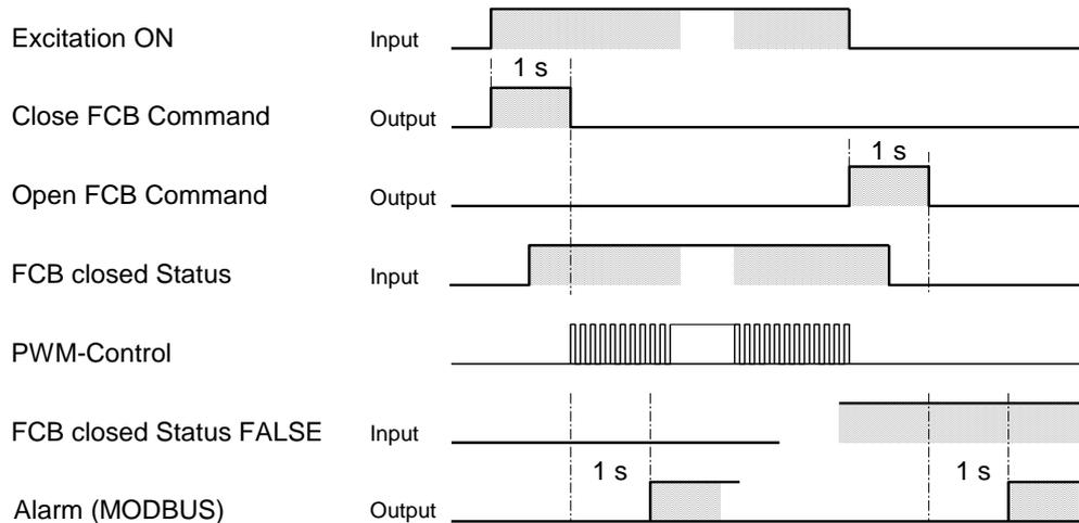
In redundant channel operation the FCB closing works as follows:
