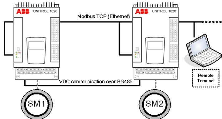
Figure 3-4 ABB solution if both Remote Access and VDC features are required.
