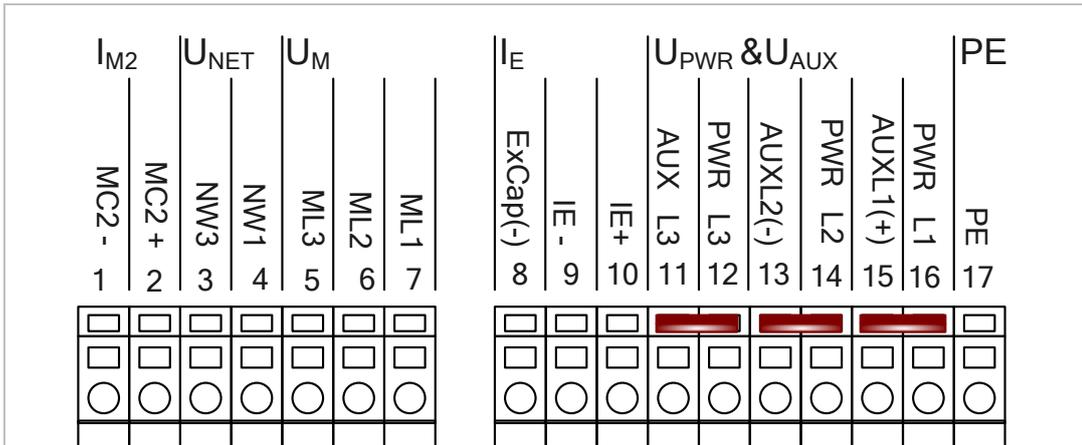
Jumper will short-circuit power input with auxiliary input
