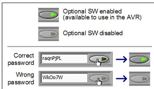
Figure 6-17 Upper: LED is bright when the optional SW is enabled in the AVR. Lower: A wrong password does not enable the SW.
