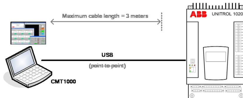
*Figure 3-2 USB connection to a PC*
