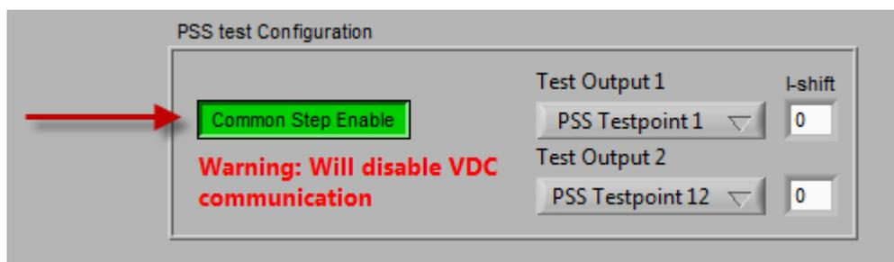
If the *Common Step Enable* button is selected, this status is shown in the setpoint adjust window (indication turns green).
