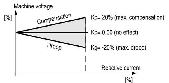
The second droop setting can be selected by digital input or over Modbus. Droop setting can be selected on active power as well.
