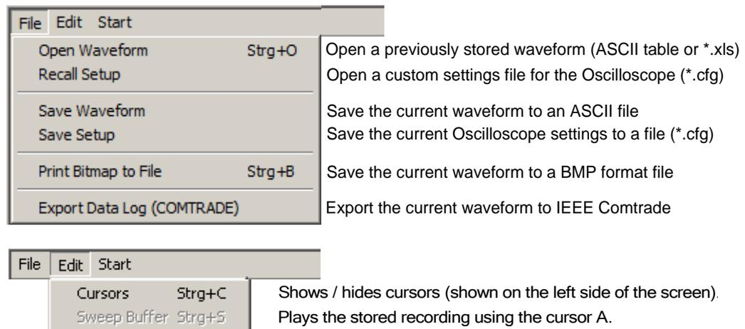
Figure 6-20 Menu structure of the Oscilloscope tool window and function of each item.
