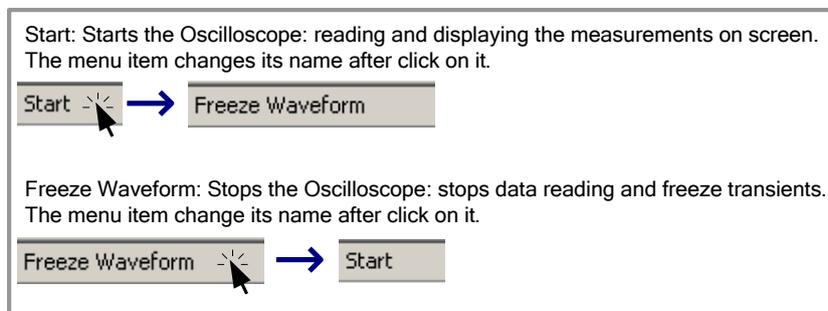
Figure 6-21 The Oscilloscope is started and stopped using the "Start" / "Freeze Waveform" button located in the menu of the window.
